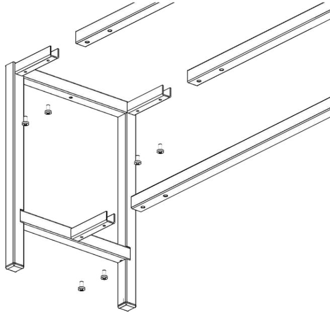
2. Encaixe as travessas(2) no Pé Central(4) e fixe com parafusos M6x12(B)
